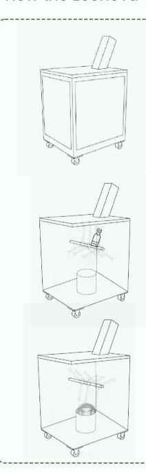
Load the Glass Waste: Insert glass bottles, jars, or other glass waste into the hopper. The wide-mouth design ensures smooth and easy loading.
