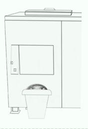
**Waste is Added :** Organic waste is loaded into the machine, and the process begins by pressing the start button on the touchscreen.
